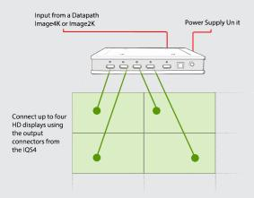
Outputs from the IQS4 can be connected to any four screens on the wall, the DDCT will work out the correct configuration.
