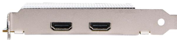
\* Note: It is recommended that only authentic cables, approved and certified by HDMI are used with the VisionSC-UHD2 card. When capturing 4k 60p, Premium Certified cables should be used.
